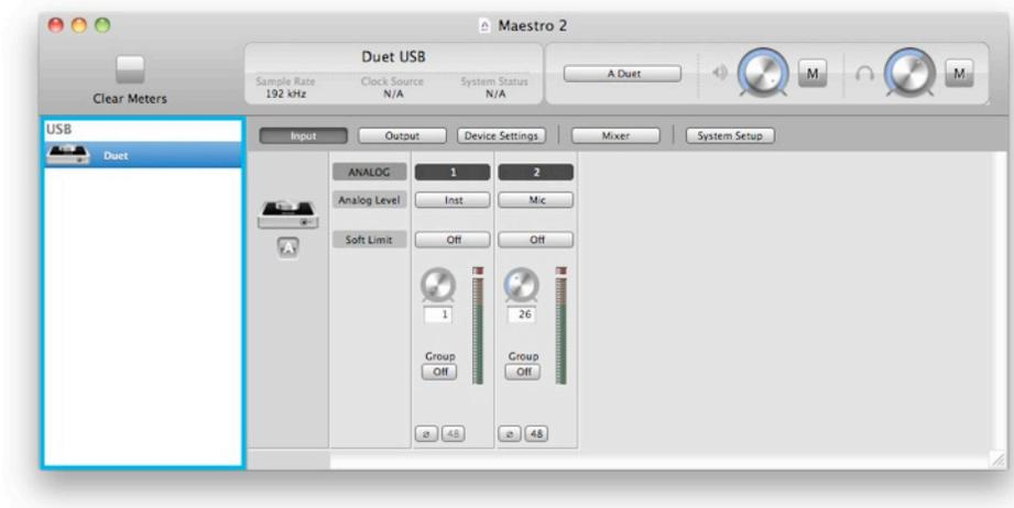
Any Maestro-compatible Apogee interfaces connected to the host computer are displayed in the Devices sidebar, regardless of whether the connection is made via Symphony PCI card, USB or FireWire. Hardware settings are displayed by first selecting one or more interfaces in the Devices sidebar and then clicking on a tab.
