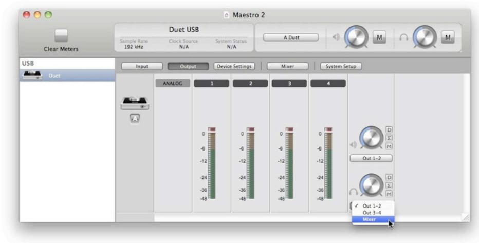
After making the input selection and setting gain, the signal should be displayed on both the Input and Mixer Master meters. If the Input's Over LED lights, reduce the input gain in the Maestro Control window. If the Mixer Master's Over LEDs light, reduce the Input fader.
