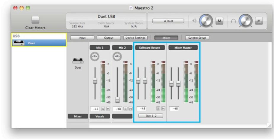
Now start playback in your recording software. The playback signal should be displayed on the Software Return and Mixer Master's meters. Use the Software Return and Input faders to establish your desired balance between the input and playback signals. If you've found a good balance but the Mixer Master's Over LEDs light, reduce the Mixer Master fader.
