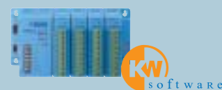
ADAM-5510KW: 4-slot PC-based SoftLogic Controller
