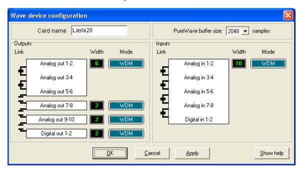
*Mode button:* The blue mode buttons let you set either WDM or PureWave mode for each individual wave device. Just click the button to change the mode.
