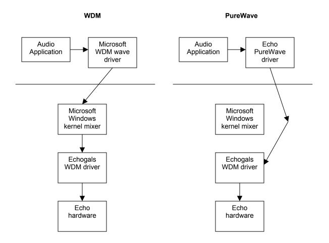
As you can see from the diagram, PureWave mode completely bypasses the Windows kernel mixer to deliver your audio data directly to the hardware.
