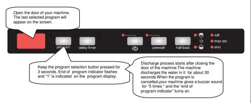
**Note:**When the door of the machine is opened in order to stop the washing program before it is completed first open the door slightly in order to avoid water spillage.
