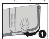
Push the latch to open the detergent container as shown in the image. 1 Detergent pod has level lines inside. It is possible to measure the right detergent amount using these lines. Detergent pod can take totally 40 cm³ detergent.
