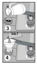
machine. Otherwise, the function of the softener compartment may decrease over time. When you start your dishwasher, the salt compartment gets filled with water. Therefore, put the softener salt prior to starting your machine.
