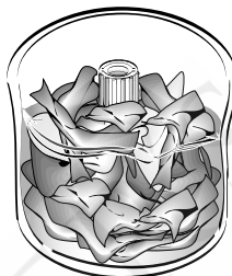
Wrong Water Level for Size of Load
