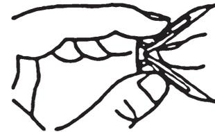
Fig. 8 - Popping Open Anchor Wing For Thin Walls
