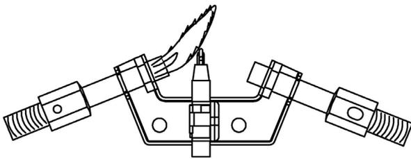
Fig. 21- Incorrect Pilot Flame Pattern
