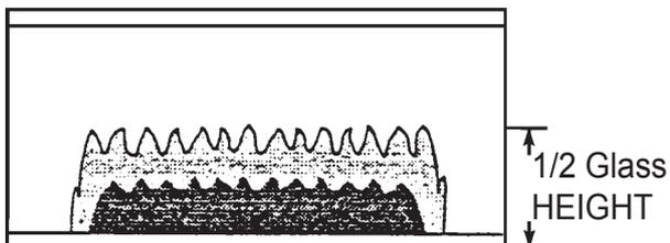
Fig. 23 - Incorrect Pilot Flame Pattern with Control Knob Set to High Flame (5)
