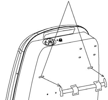
Fig. 10 - Installing Bottom Mounting Bracket
