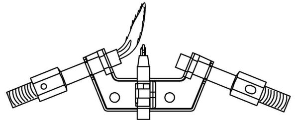
**⚠ WARNING:** If yellow tipping occurs, your heater could produce increased levels of carbon monoxide. If burner flame pattern shows yellow tipping, follow instructions at bottom of this page.
