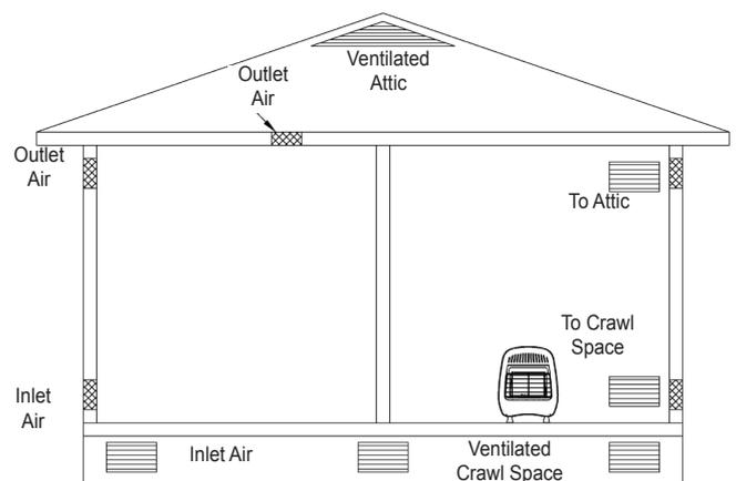
**IMPORTANT:** Do not provide openings for inlet or outlet air into attic if attic has a thermostat-controlled power vent. Heated air entering the attic will activate the power vent. Rework worksheet, adding the space of the adjoining unconfined space. The combined spaces must have enough fresh air to supply all appliances in both spaces.
