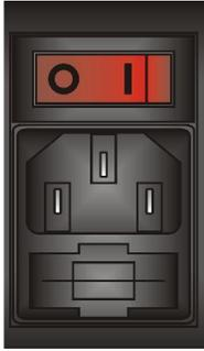
The Falcon 15 uses a power entry module with AC switch just closed to the IEC power cord receptacle. It can operate on 110 or 240 VAC, 50/60 Hz AC mains voltages. If the unit is to be used with a mains voltage different to that for which the unit is supplied, set the voltage change-over switch, which is placed inside the box, closed to the AC transformer.
