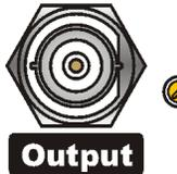
Depending on the version, Output BNC connector (50 Ohm impedance) features Stereo Composite Signal (MPX) and/or RDS signal (with or without signals injected from Aux 1 and 2 mixed into).
