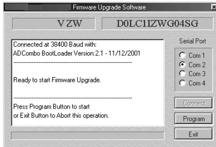
**K)** Make sure the Identification is correctly done (*Ready to start Firmware Upgrade* message + firmware code displayed in the right field), and click '**Program**' button. The upgrade will continue automatically.
