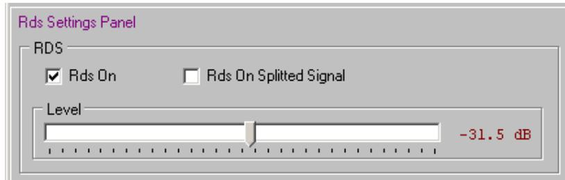
You may also switch RDS generation on and off and enable/disable RDS output while the Falcon 15 FM is on split (i.e. while it is replicating an external MPX signal on its output).
