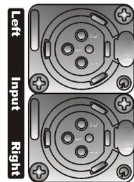
Balanced XLR-type connectors are used for input analog audio.
