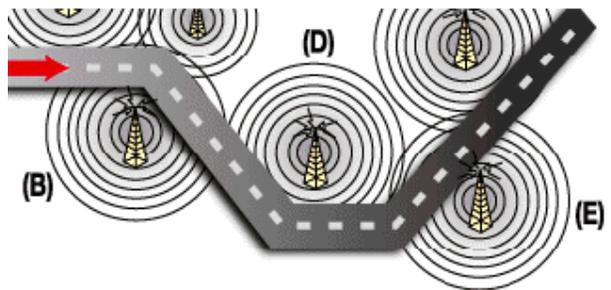
Returning to the example of transmitters B, D and E in the previous paragraph (in which the coverage areas of D and E do not overlap), two more lists will be assigned to transmitter B, sorted according to the above criteria to take into account any different programming by some of the AFs.
