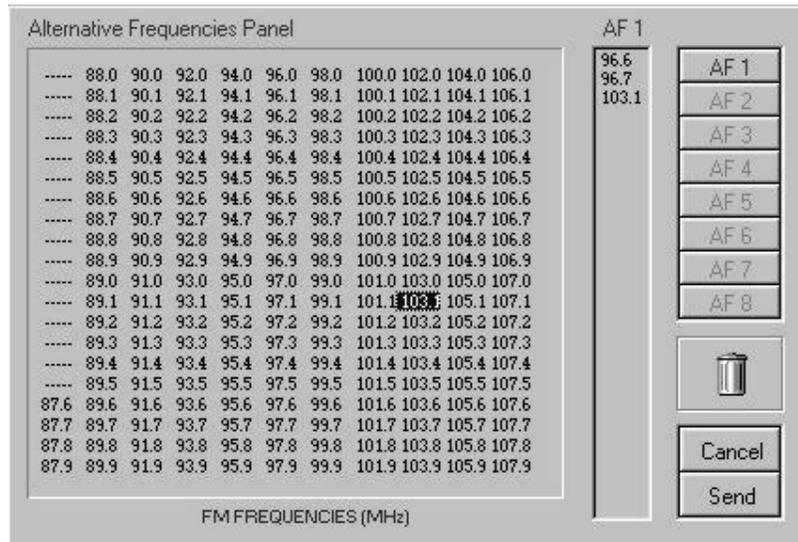
The list(s) of **alternative frequencies** give information on the various transmitters broadcasting the same programme in the same or adjacent reception areas, and enable receivers equipped with a memory to store the list(s), to reduce the time for switching to another transmitter. This facility is particularly useful in the case of car and portable radios.
