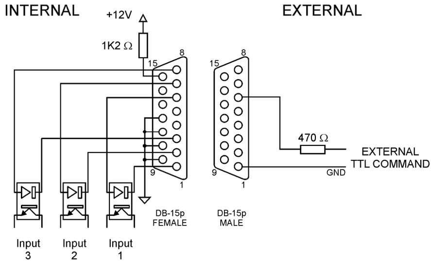
Apply an external TTL signal through a 470 Ohm carbon resistor to the photodiode 1 (pins 6 and 1). Max current allowed: 10 mA. Nominal: 5 mA
