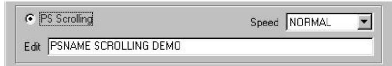
PS Scrolling panel allows You to enter PS message which will scroll on the receiver display. It means, text is moved right to left across the display one character at a time at the rate set by the user (SPEED).
