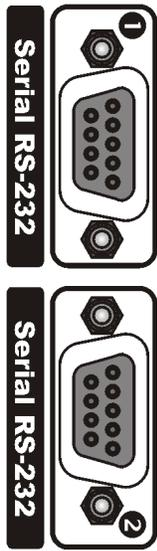
Falcon 15 features up to four optoinsulated RS232 serial ports (port 3 and 4 are available as an option) which allow the remote control and RDS programming both through local - or remote PCs, UECP programmer, etc.
