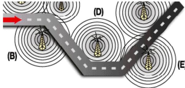
For example, in the situation shown in the figure three transmitters (B, D, E) intersect only in two coverage areas: between B and D, and between D and E. The following lists should be loaded in each transmitter:
