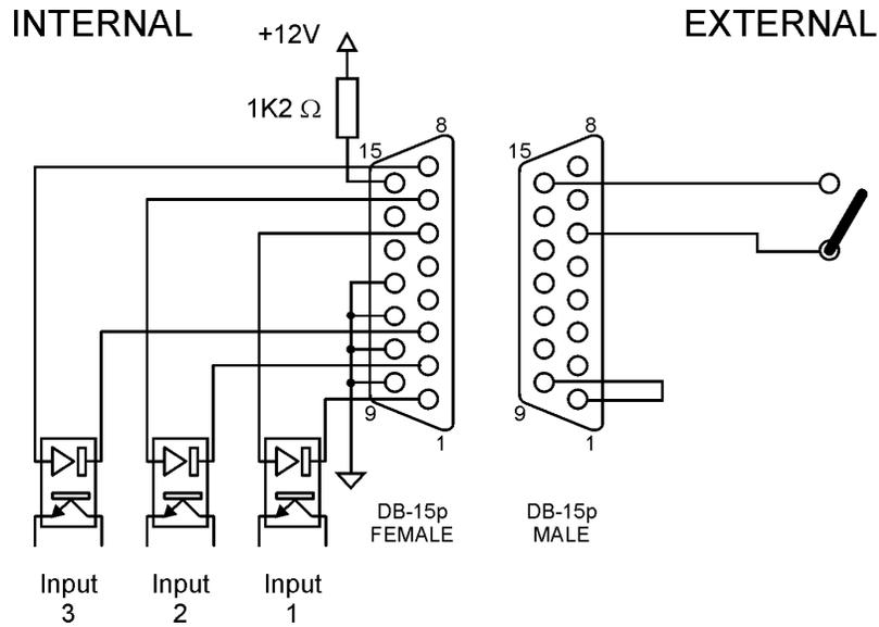
shortcut pin 9 and 1 and shortcut pin 15 and pin 6 via an external switch.
