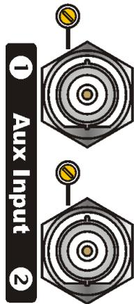
The Aux inputs allow the Mpx, SCA, RDS injection from external coders. The resultant signal (f.i. external RDS+ self-generated MPX) is available on the **Output** connector.
