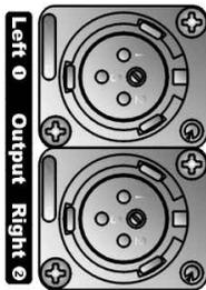
Balanced XLR-type connectors are used for output analog audio. The stereo analog outputs are designed for standard 0 dBu (line- level) balanced signals. Output level setting is done using the software parameter settings (see par. 14.3).
