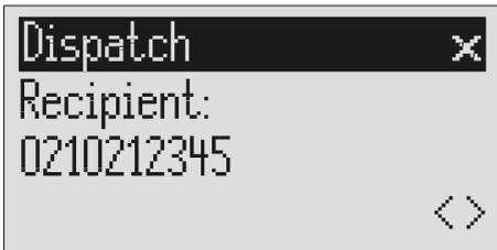
Enter the first digit of the call number using the control buttons (up/down).
