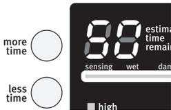
When you select a Timed Cycle, the default time appears in the display. Use the More Time/Less Time buttons to increase or decrease the time in 1 minute increments. Press and hold to change the time in 5 minute increments.
