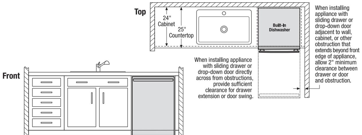
When installing appliance with sliding drawer or drop-down door directly across from obstructions, provide sufficient clearance for drawer extension or door swing.
