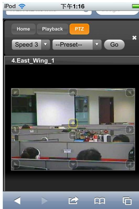
**Fig. 19 Live streaming with PTZ control**
