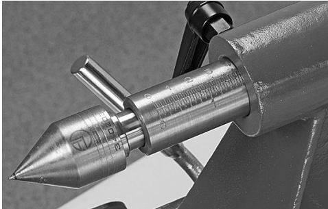
Tailstock barrel with scale
