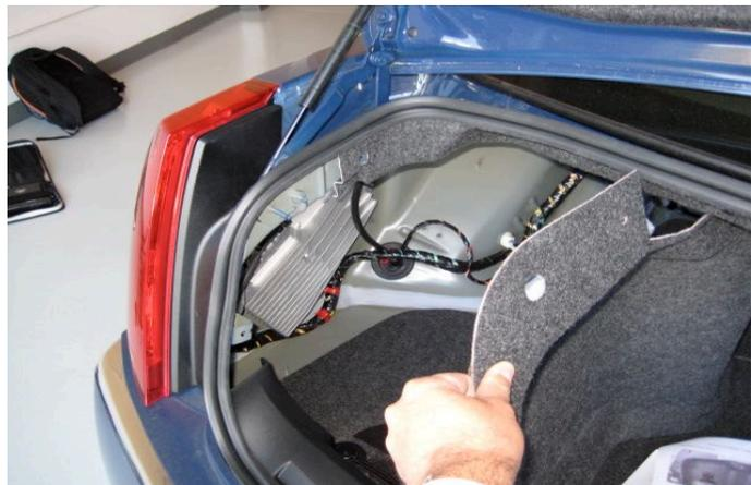
5. Using Router Docking Station as a template, drill or punch four 1/8" diameter holes in level area near rear of trunk liner. Use caution-insulation located behind this area can bind in drill bit.
