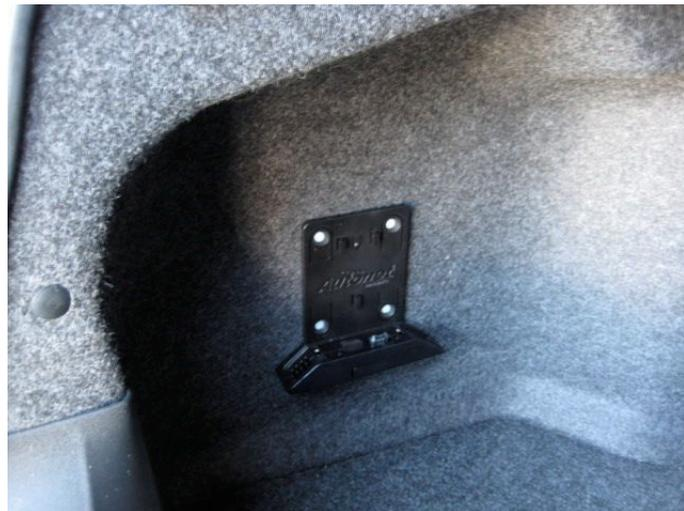
7. Drill a 3/8" hole directly below docking station for power wire.
