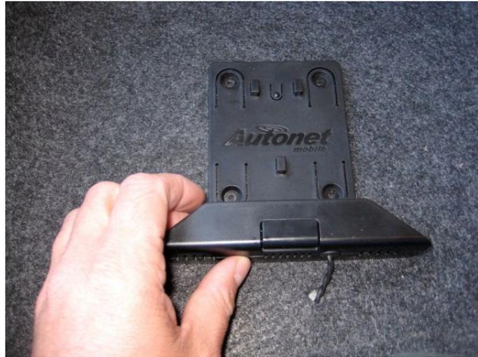
6. Attach docking station using four supplied nylon Key Hole clips.
