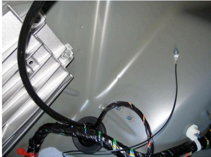
10. Feed cable through seat frame into passenger cabin.
