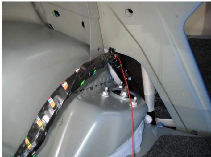
11. Run power cable under trim to left instrument panel access area on the driver's side of dash.
