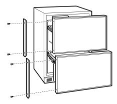
3. Custom handles of your choice, supplied by your cabinet maker, must be installed onto the overlay panels before they are slid into the trims. Countersink all screws into the backer panels. Screws cannot protrude from the backer panels.
