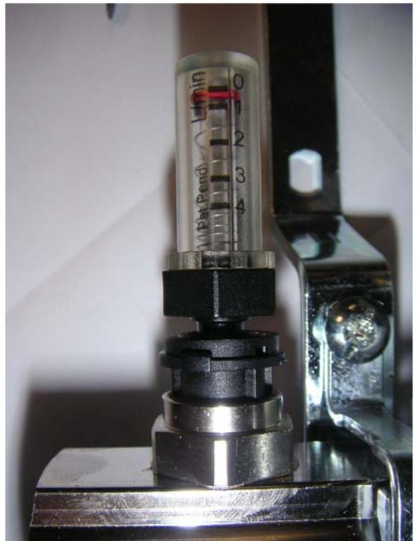
**Step 3** Push the white cap to the base of the flow meter so it clicks down as in fig 34 below.
