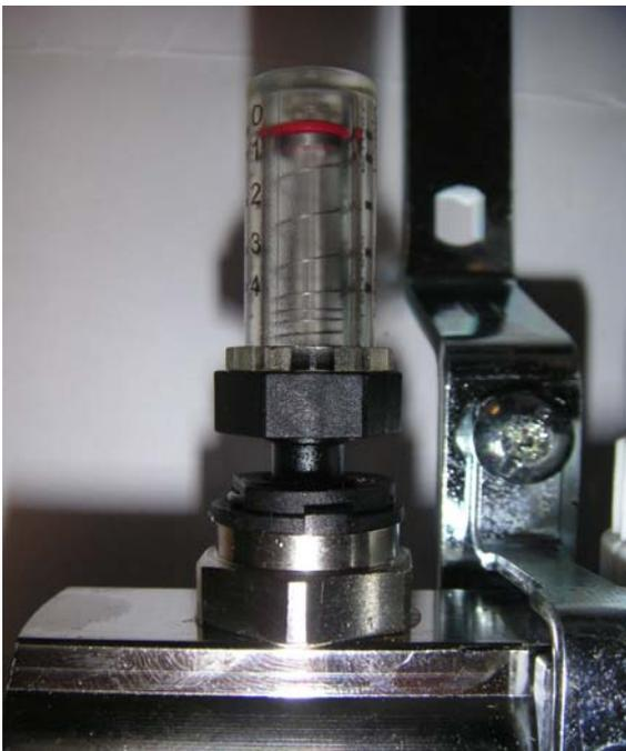
**Step 2** Use the white cap to turn the whole flow meter anti-clockwise until the flow meter is open. (Alternatively, use a pair of grips)
