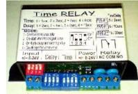
Fermax IP DP panels can be equipped with an additional time switch called "TimeRelay". It is used for an expansion of the number of switches. It is programmable. Based on switching of one of the two switches in the Fermax IP DP panel, the TimeRelay can simulate e.g. sequent opening of the door or alternatively you can connect the exit button.
