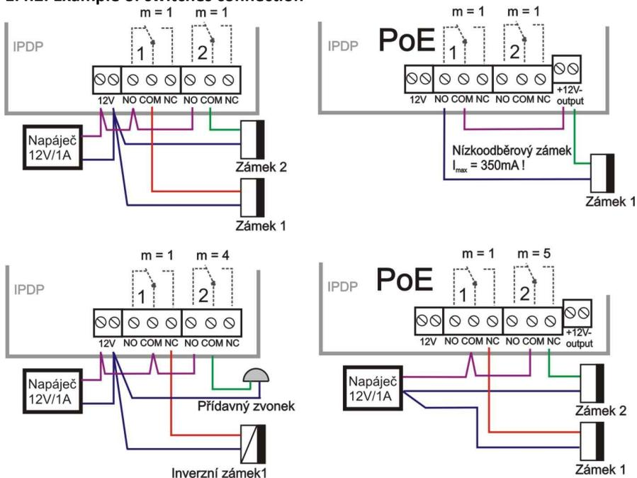
The switching contact of relay is separated galvanically from other circuits of the door phone panel.
