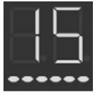
The numerical LED display usually shows the current preset number. When the GUITAR layer button is pressed, the LED will show the sound mapped to the GUITAR layer for a few seconds, then revert to the preset number. This functions the same for all the parameter buttons.
