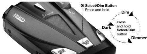
**To Set the Display Dim Mode Default Directly Using the Set/Dim Button**
