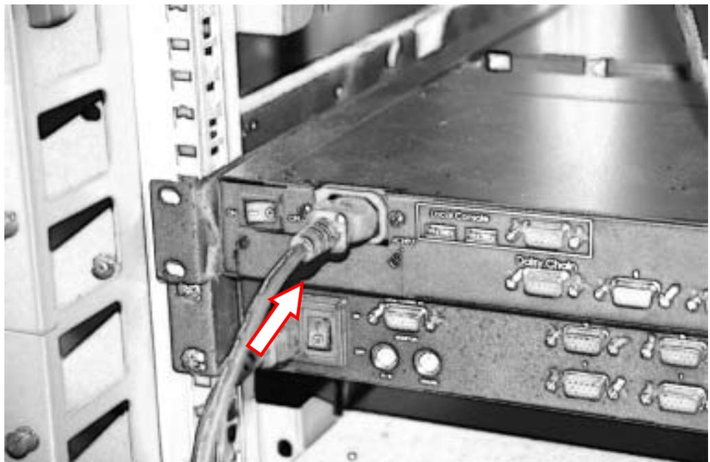
2.5 Connect the host cable to the rear of the drawer. For the 920, USB type can be connected to its single port. For 980/990 both PS/2 and USB type can be use with the KVM, just choose the desire type to match with your system, the KVM accepts both. Refer to **Section 3** for further detail. (\*980 Shown)
