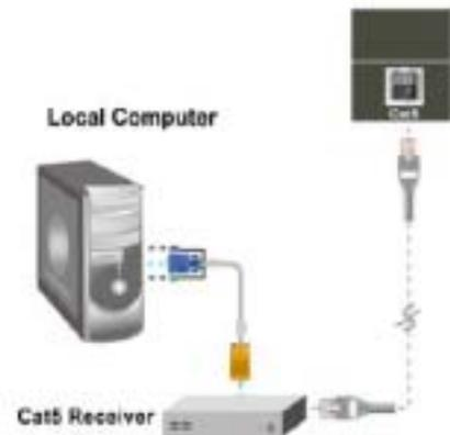
3.7 **Optional IP Remote Console Module Available** for allow redirect of keyboard, mouse and mouse data to a remote administration console. It allows you to control one or many computer locally at the server site or remotely via the Internet using standard browser.
