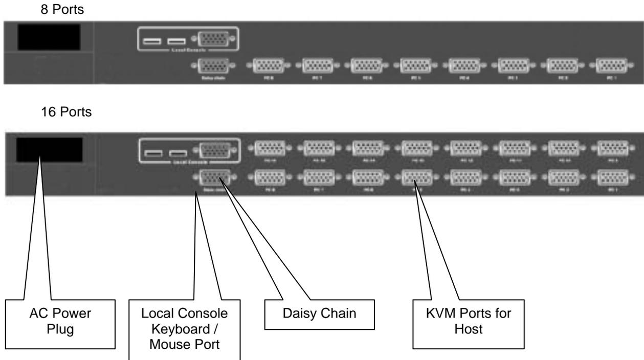
3.2 Connecting KVM Ports for Host using PS/2 connection. Connect single ended D-Sub end to KVM port and other end composing of VGA D-Sub, PS/2 Keyboard (Green) and PS/2 Mouse (Purple) to corresponding ports on the system.
