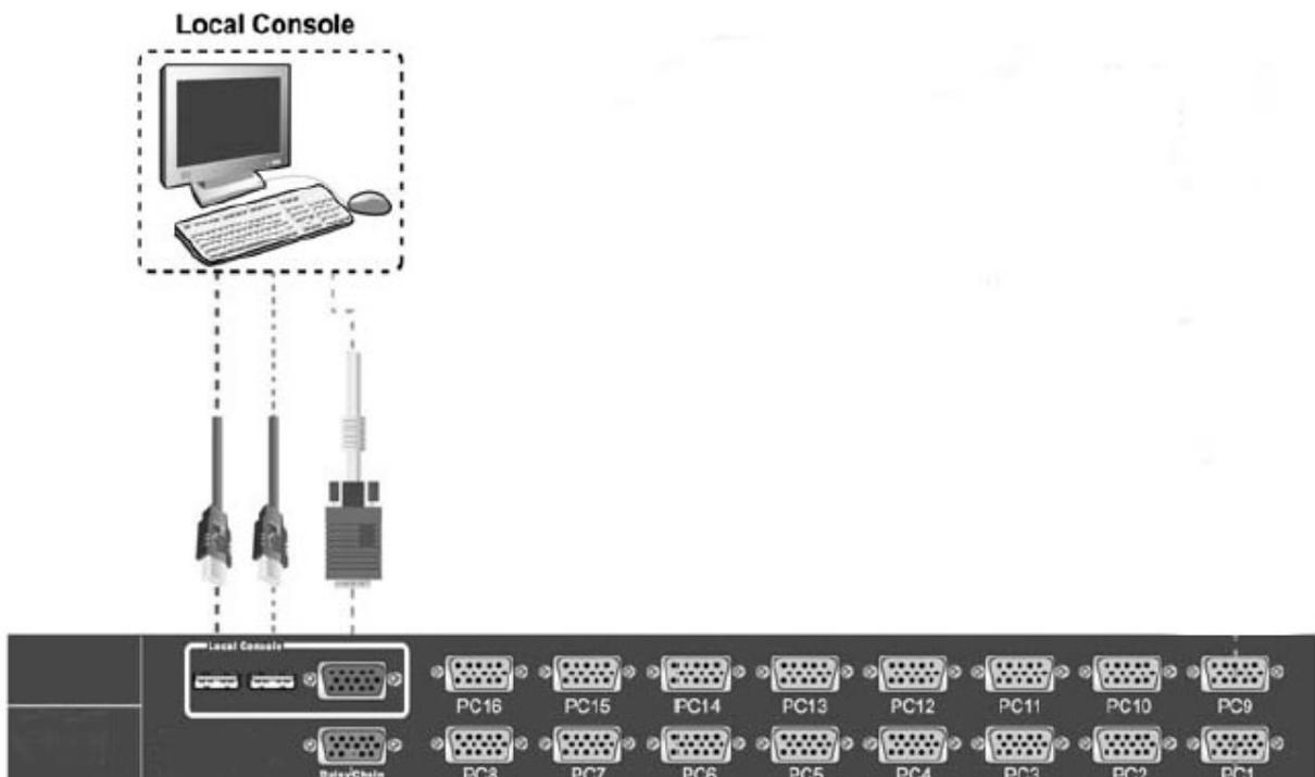
3.5 You can connect additional KVM port by adding additional KVM switches and connecting between them a daisy chain cable. The control will be from the primary KVM by changing banks selection.
