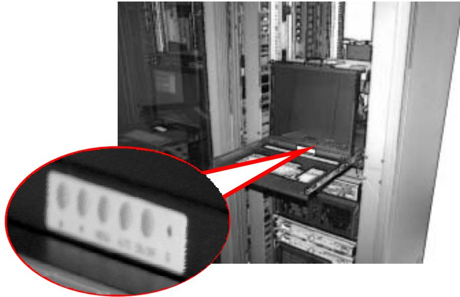
2.10 To return the drawer back to the unit, fold screen down and push in the 2 tap located on each side of the rail then push the drawer back in.
