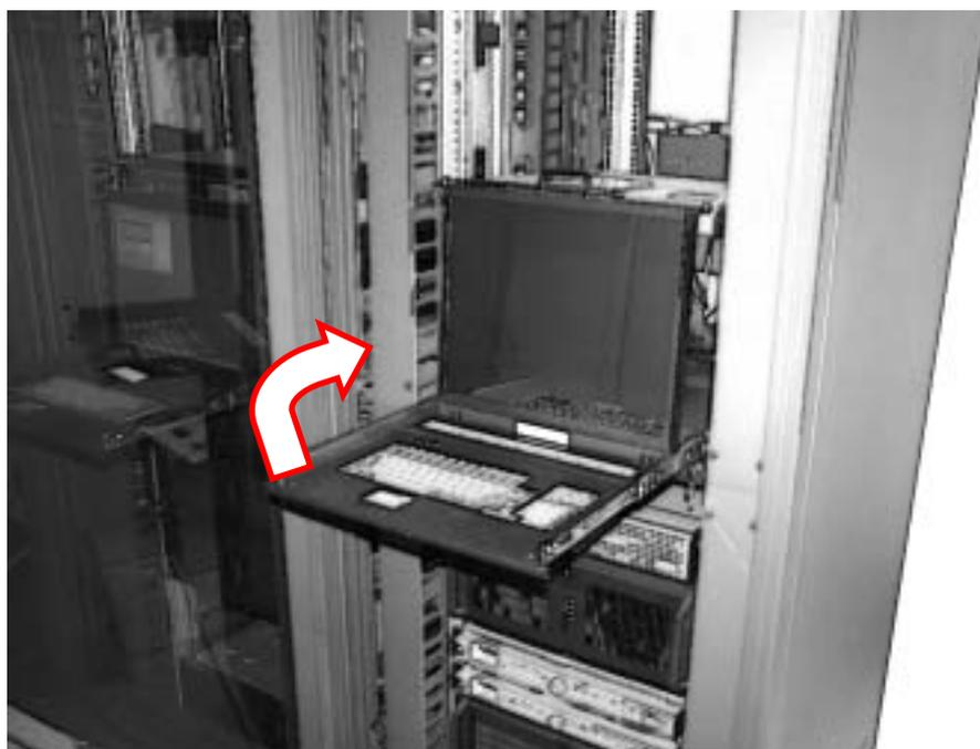
2.9 To turn on the power for the LCD panel, the power button located beneath the LCD can be used to independently turn on/off. LCD screen adjustment button is also located here.
