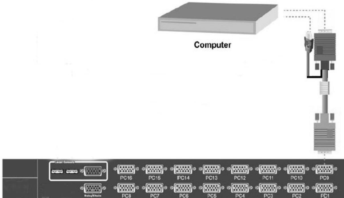
3.4 You can connect a local console port to operate the KVM bypassing the built-in LCD and keyboard/touchpad through the rear local console port. Connect the VGA D-Sub connector and USB keyboard and USB mouse to the port marked.
