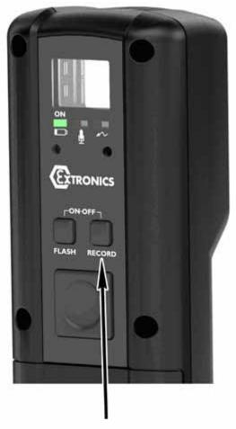
Press the "RECORD" button to enable the recording feature of the camera.
