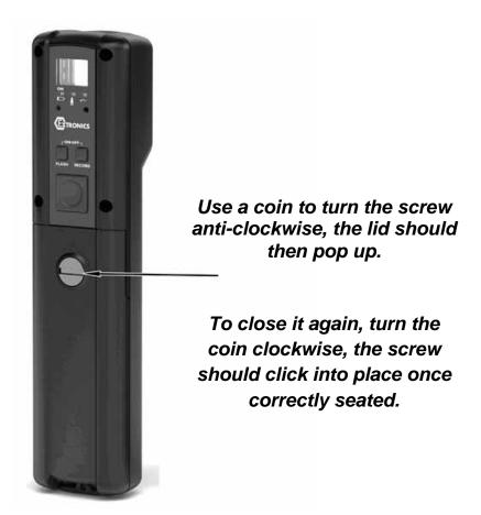
Install the batteries in the correct orientation (indicated on the enclosure) and close the lid again.
