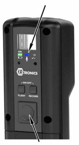
Press and <u>HOLD</u> trigger button, <u>WAIT</u> until blue LED begins to flash, then record audio and release trigger button when finished
