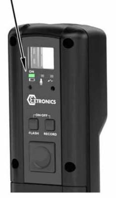
The diagrams above show how to power on the iCAM501U. The same procedure is required to turn the iCAM501U off. Once it is turned off no LED's should be lit.
