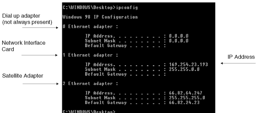
Figure 11: Displaying Ethernet adapter addresses using the ipconfig command
