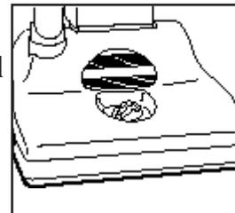
Do not adjust vacuum cleaner too low in deep pile or shag carpet. This can overload motor and damage rotating floor brush or drive belt.
