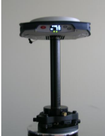
UHF Antenna ( \frac{1}{4} wave) inside the base pole extension
