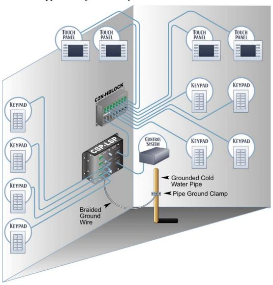
KEYPAD TOUCH PANEL KEYPAD CONTROL SYSTEM Grounded Cold Water Pipe ♣ Pipe Ground Clamp
