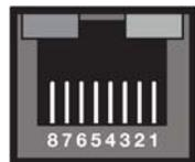
FIG. 4 Ethernet Pin Numbering
