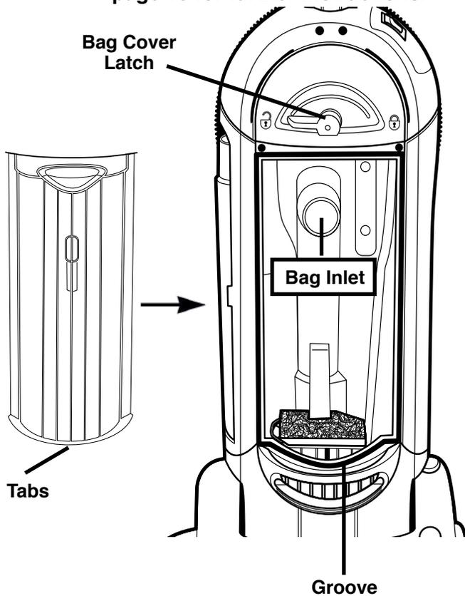
4. Replace front cover by aligning tabs at bottom of front cover into groove on cleaner. Pivot front cover up against cleaner and rotate the bag cover latch to the right to secure.
