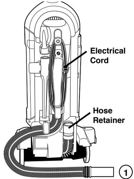
1. Remove hose from hose retainer and check suction at end of hose.
