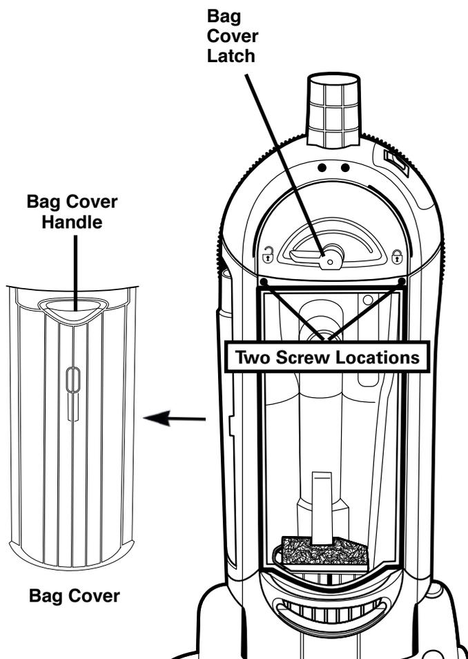
1. Remove bag cover from unit to expose the two screw installation locations. Release the bag cover by rotating the bag cover latch to the left. Pull out and up on the bag cover handle to remove bag cover from unit.
