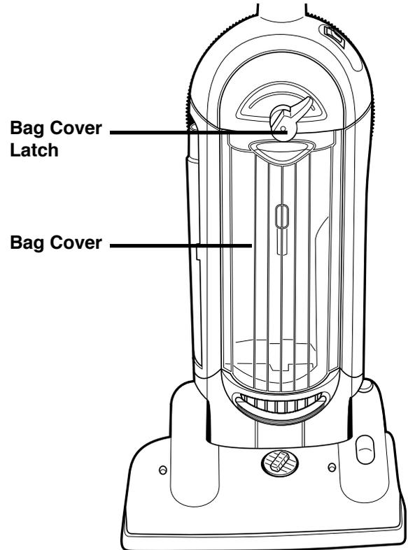
1. Release bag cover by rotating bag cover latch to the left pointing to the unlock symbol (🔓). Pivot bag cover away from cleaner and remove.
