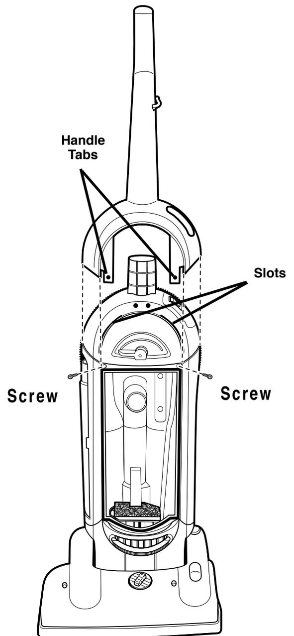
2. Position handle as above. Slide the handle down over the top of the unit, inserting handle tabs into slots on unit.
