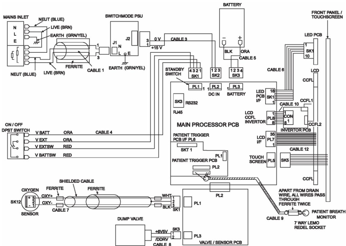
Figure 8 - IFSD Electrical Wiring Diagram
