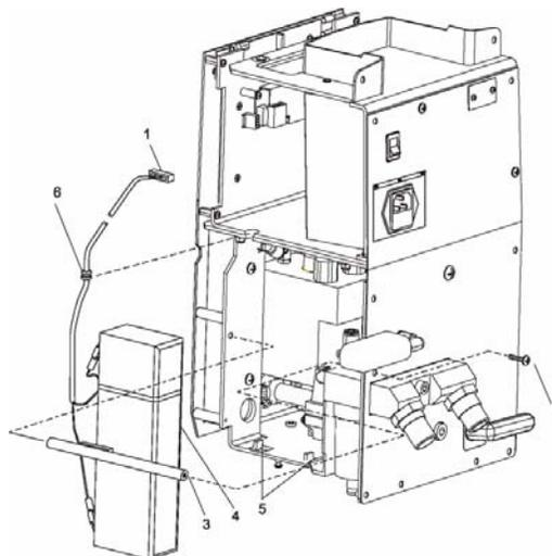
Figure 13 - Battery Removal/Fitting
