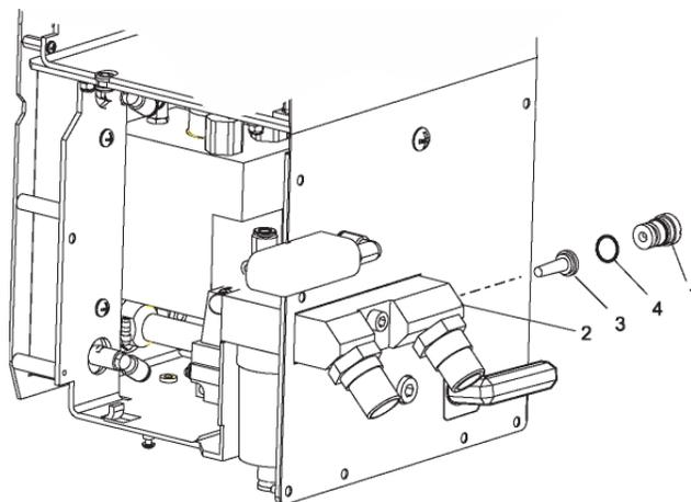
Figure 14 - Oxygen Filter Removal/Fitting
