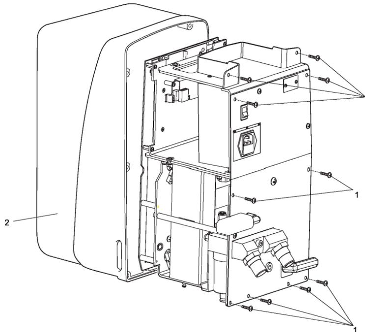
Figure 12 - Case Removal/Fitting
