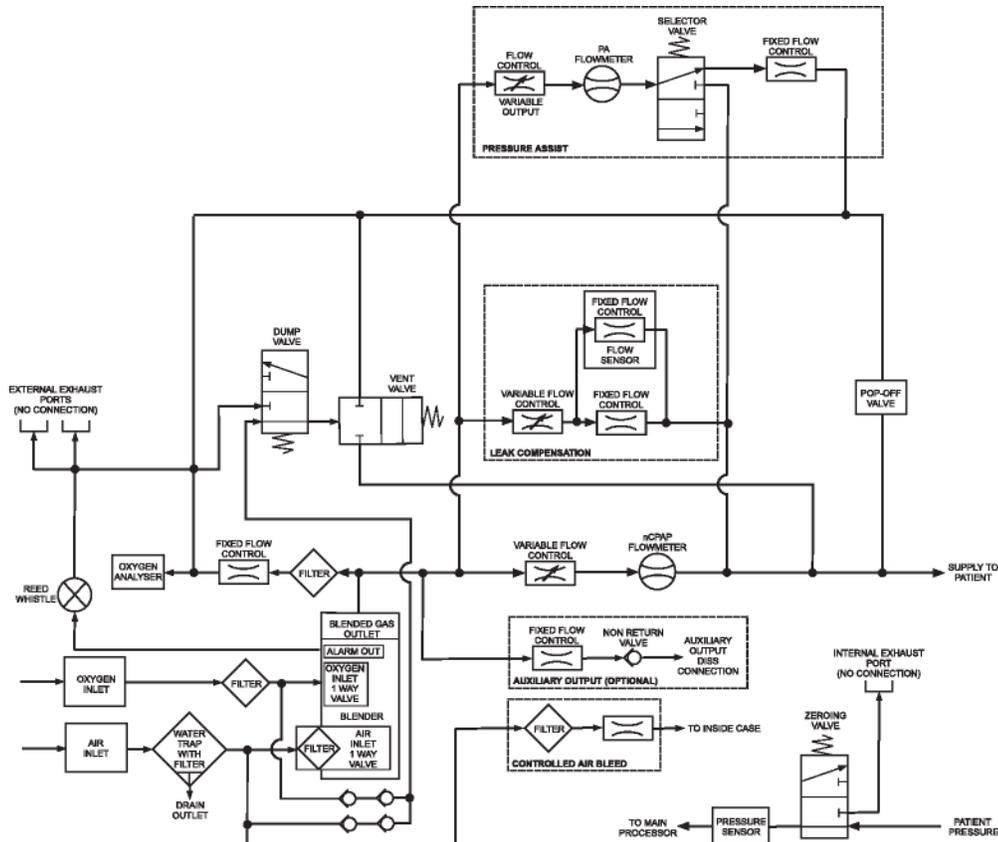
Figure 6 - IFSD Gas Flow Schematic
