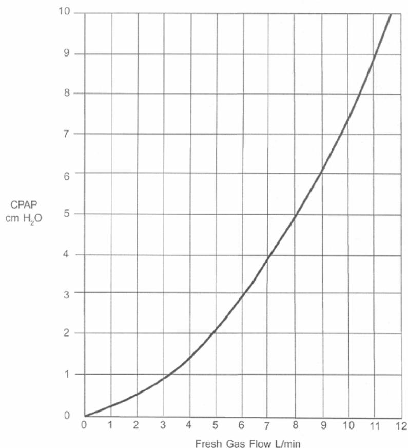
**Figure 10 - Flow Pressure Nomogram**
