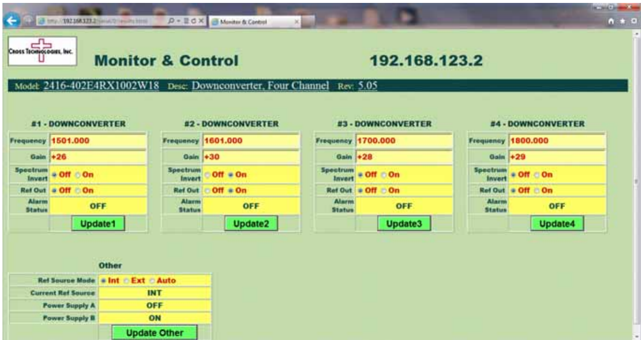
Figure 3.3: Model 2416-x02 Web Page (Example above shows M&C Web Page for Model 2416-402)
