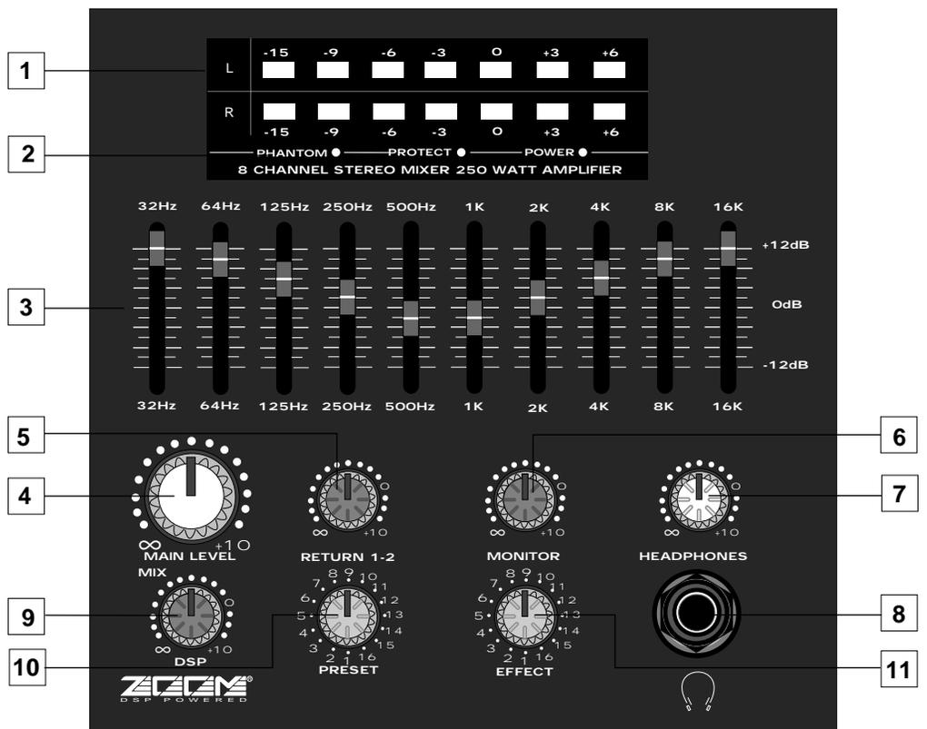
**1: Meter** - This seven-segment bar meter shows the continuous output level of the SD8. For optimum signal-to-noise ratio, try to adjust all Levels (channel and main) so that program material is usually at or around 0 VU, with occasional but not steady excursions to the +3 segment. See the “Setting Up and Using the SD8” section on page 12 in this manual for more information.
