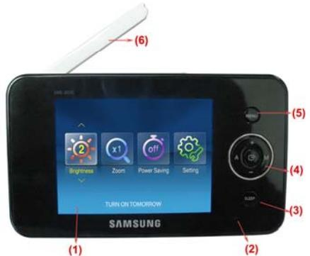
**4. Navigation Controls/OK Button** – Use the controls to move and select while in Viewing Mode and Menu Mode.
