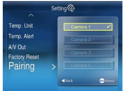
4. Select a channel by pressing the **[+]** and **[-]** keys. Press the **OK** button on the receiver to accept.
