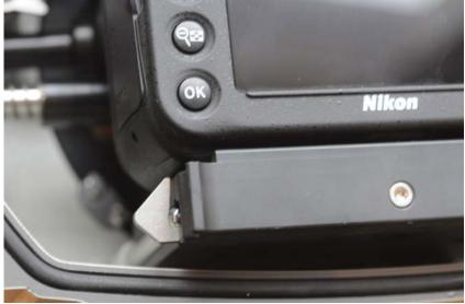
Insert the synch cord connector in the direction indicated by the arrow on the top of the connector into the camera hot shoe (the cable pointing into the housing). – if fitted
