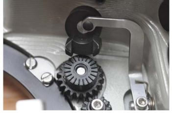
Turn the focus coupler lever down to **AF** position. This moves the crown wheel inside the housing outwards and makes loading the camera into the housing easier, and is necessary in any case if a zoom or focus gear is used on the lens.
