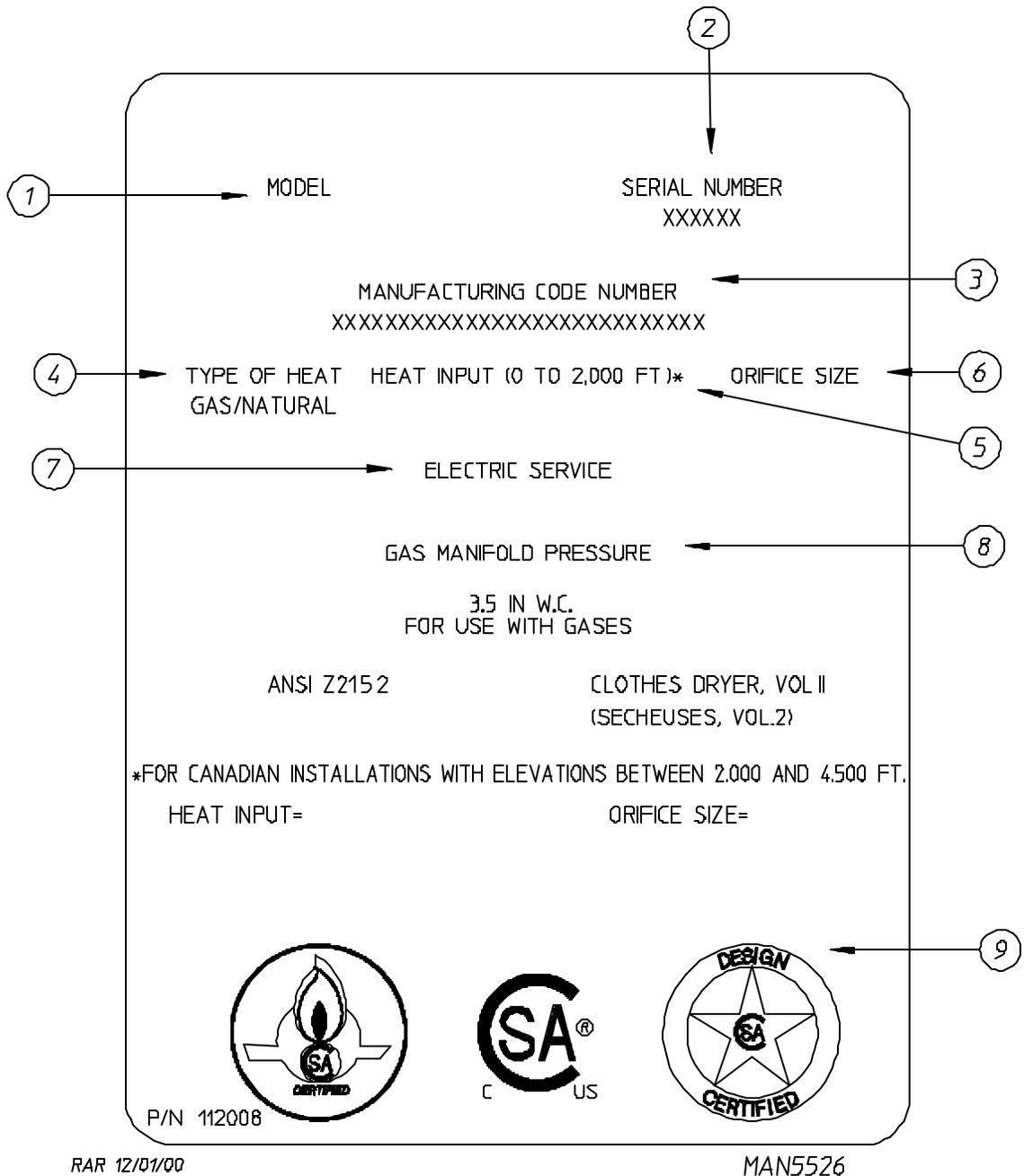
When contacting **ADC**, certain information is required to insure proper service/parts information from **ADC**. This information is on the dryer data label affixed to the back panel of the main electrical cabinet located in the right hand electrical enclosure. When contacting **ADC** please have the **model number** and **serial number** available.
