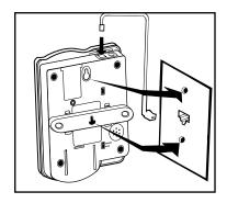
Fig. 6 - Wall mounting installation.
