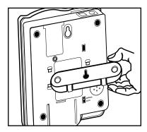
Fig. 5 - Phone base installation for wall mounting
