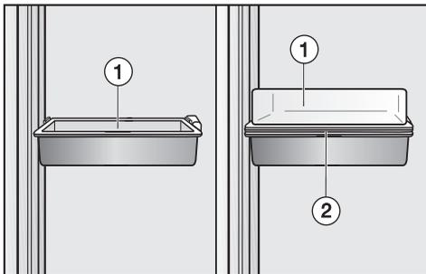
It consists of a deep tray ① and a shallow tray ②. Both trays fit the stainless steel frame.
