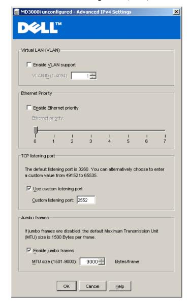
Figure 11: MD3000i Advanced IPv4 Settings: VLAN, QOS, Jumbo Frames Support
