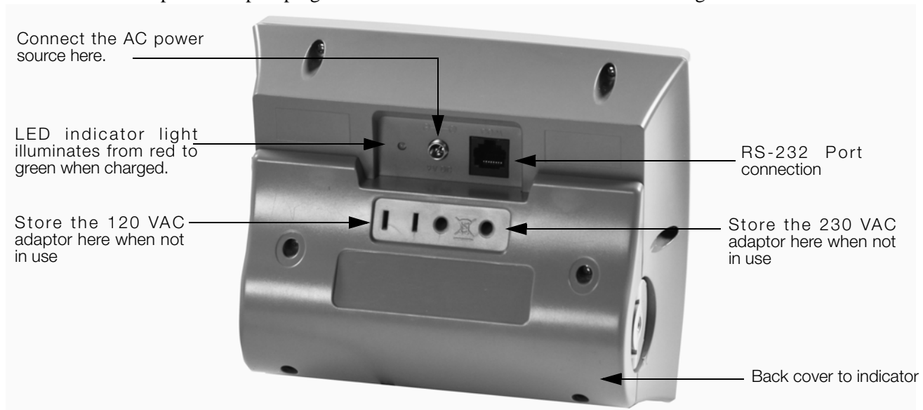
Figure 2-1. LED Light Location
