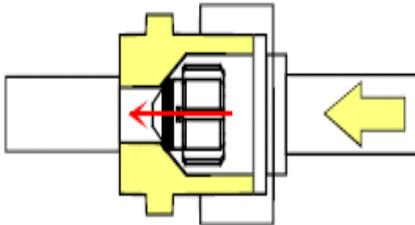
In the cooling mode, the orifice is pushed into its seat, forcing refrigerant to flow through the metered hole in the center of the orifice.
