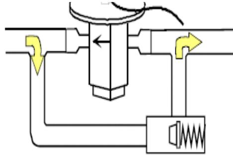
Most expansion valves used in current Amana® Brand Heat Pump products use an internally checked expansion valve. This type of expansion valve does not require an external check valve as shown above. However, the principle of operation is the same.
