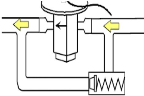
**EXPANSION VALVE/CHECK VALVE ASSEMBLY
