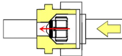
In the cooling mode, the orifice is pushed into its seat, forcing refrigerant to flow through the metered hole in the center of the orifice.
