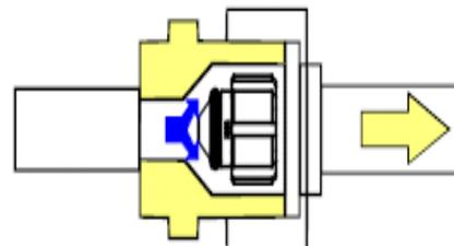
In the heating mode, the orifice moves back off its seat, allowing refrigerant to flow unmetered around the outside of the orifice.
