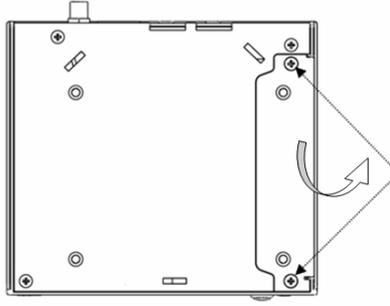
2. Slide disk in until it is connected firmly. The two hard disk screw holes should be aligned with the holes in the base.
