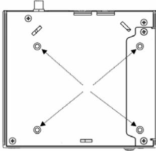
1. Open the two screws on the HDD cover indicated below and remove it.
