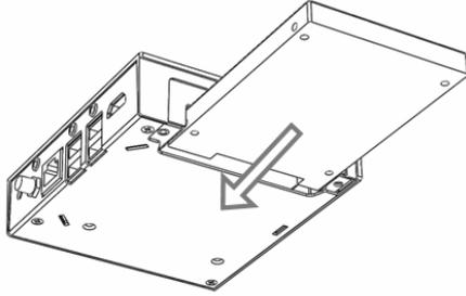
3. Replace the HDD cover and tighten the two screws.
