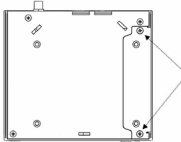
4. Tighten the four HDD screws indicated below.
