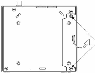
2. Flip the cover (see below) and reattach the two screws to use it as a handle to pull out the HDD.
