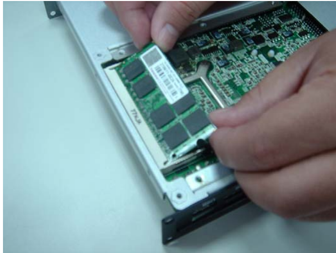
Figure 5 Fully insert the SO-DIMM Memory Module into the onboard socket
