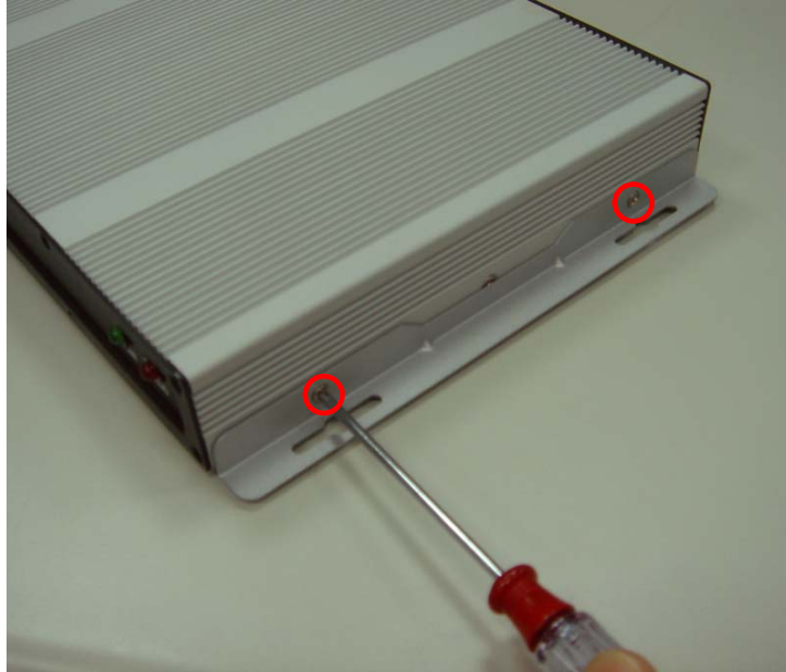
Figure 7 Secure the L-brackets for wall mounting
