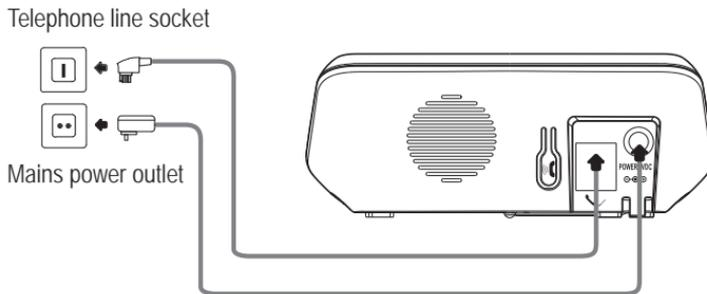
**⚠ Attention:** Use only the power adapter plug supplied with the telephone! Ensure access to the power adapter plug is not obstructed by furniture or such.
