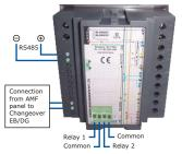
Note: Connections to the terminals located at the rear side of the unit is to be made by using preferably 12 to 14 SWG (2.6mm² to 2.6mm²) industrial grade wire. Relay rating No contact SPST. 250VAC / 30VDC @ 2 Ampsresistive.
