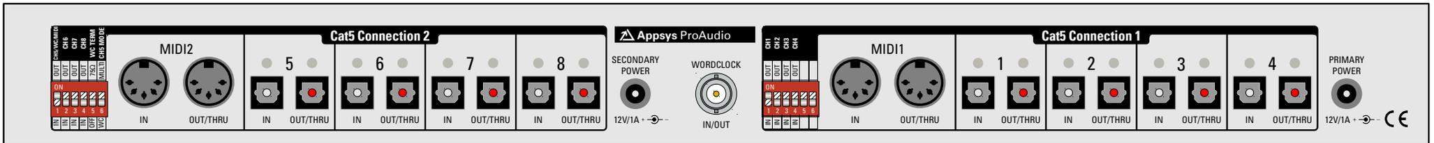
The connectors "Cat5 Connection 2" and "WORDCLOCK" are only available in the 64 channel version (ADX-64B-PRO).
