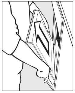
Hold the door securely at both sides, and lift it upwards off the retainers. Make sure you take it off straight.
