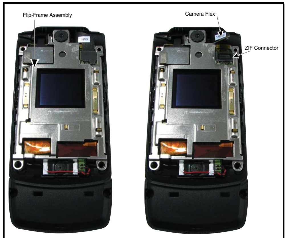
Figure 15. Camera Assembly Removal
