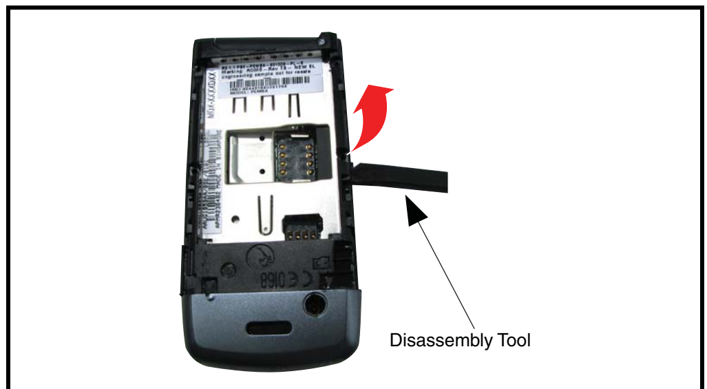
Figure 6. Removing the Rear Housing Assembly
