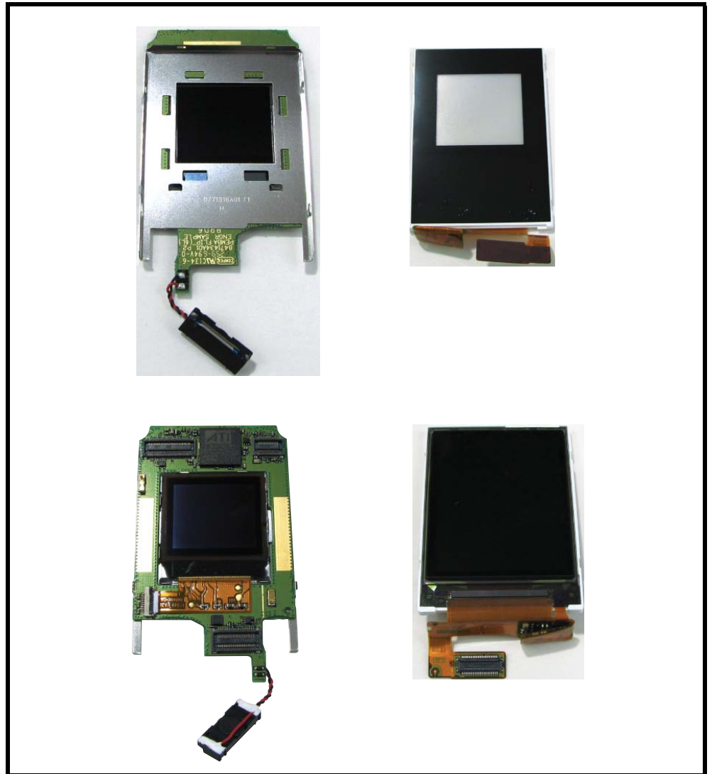
Figure 18. Removing the Display Module Lens
