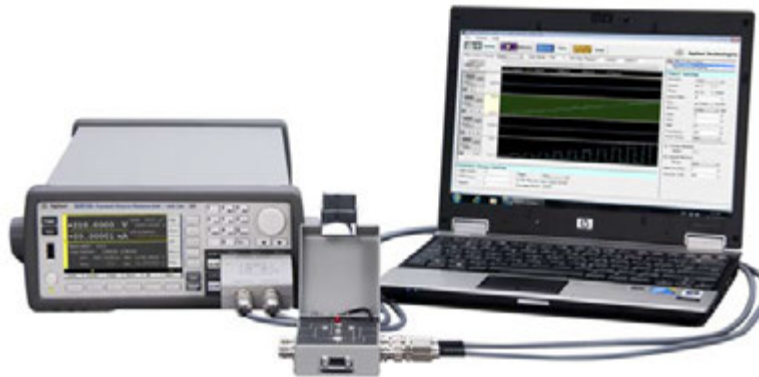
Figure 2-6 Remote control of B2912A by external PC (through USB/LAN/GPIB)
