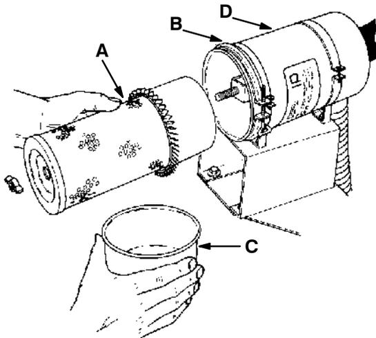
**REMOVING AIR FILTER ELEMENT**
