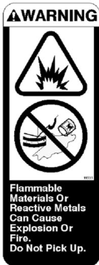
**FLAMMABLE MATERIALS WARNING DECAL - LOCATED ON THE SOLUTION TANKS**
