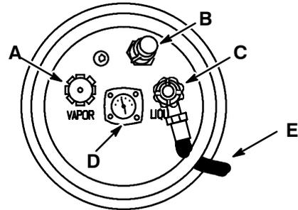
**TYPICAL LPG LIQUID WITHDRAWAL FUEL TANK** 03485
