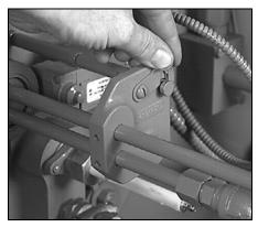
Figure 6-18 Oil Gun Locked Out
