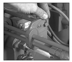
Figure 5-12 Oil Gun Locked in OUT Position
