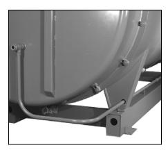
Figure 8-24 Rear Door with Site Glass Cooling Tube
