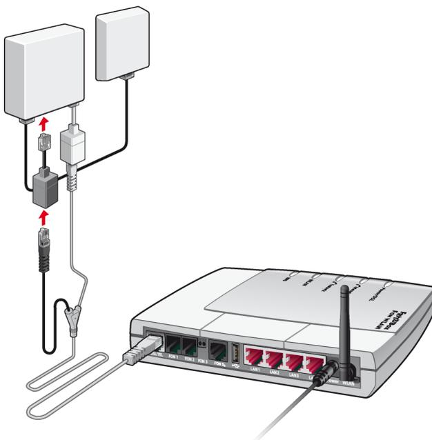
*Connecting an analog telephone line to FRITZ!Box Fon WLAN*
