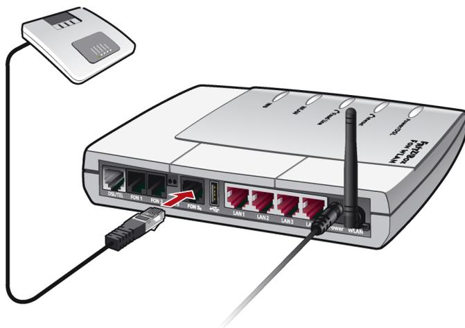
Connecting an ISDN PBX to the FRITZ!Box Fon WLAN
