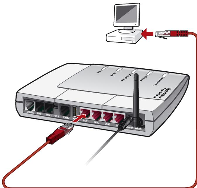
*Connecting a computer to a LAN port on the FRITZ!Box Fon WLAN*
