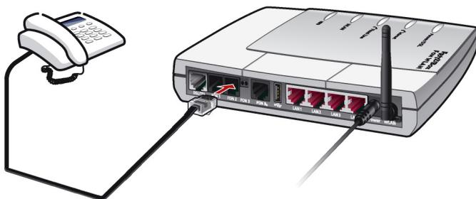
*Connecting an analog telephone to FRITZ!Box Fon WLAN*
