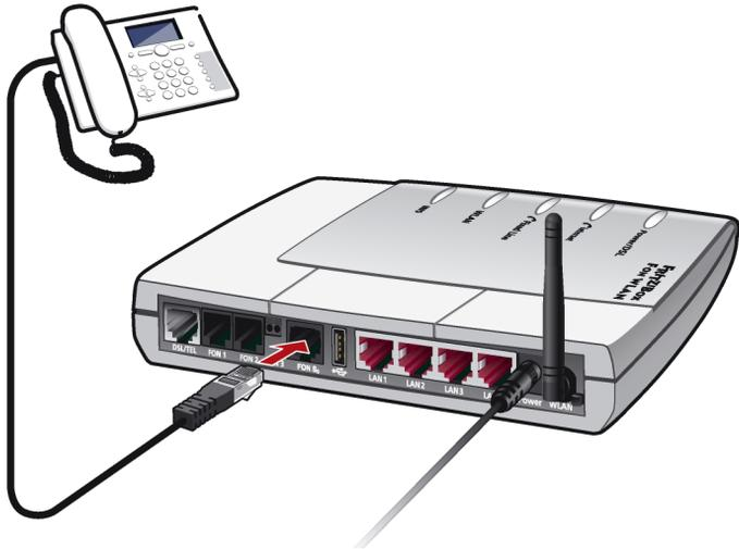
*Connecting an ISDN telephone to the FRITZ!Box Fon WLAN*
