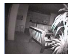
Camera in B/W mode with IR illumination on
