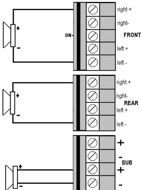
**NOTE:** The dual + and - subout terminals of the 1100.5 are paralleled internally and the combined load impedance should be taken into consideration when connecting multiple subwoofers.
